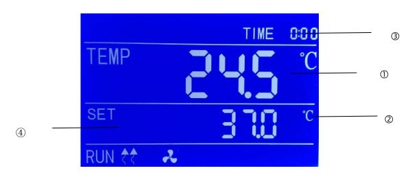
①temperature display②temperature setting③time setting④system operation status
